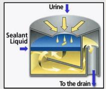
There are several waterless urinal cartridges proprietary to the urinal brand they work in. All have the same concept to function as a waterless device. When the urinal is used, urine is directed into a collection area in the center of the cartridge as shown in the image to the left.
