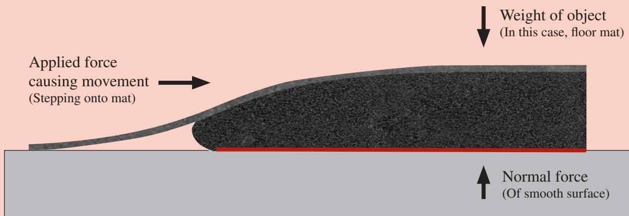
Mat movement or slippage is tested and evaluated based on its Coefficient of Friction (COF). Coefficient of friction measures the ratio of the force of friction between two bodies and the force pressing them together. The coefficient of friction depends on the materials used; for example, ice on steel has a low COF, while rubber on pavement has a high COF. Coefficients of friction range from near zero to greater than 1 (the greater the number, the higher degree of friction or slip resistance).
