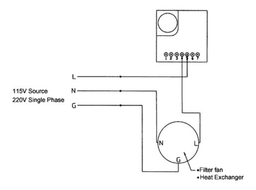
3110 Thermostat, wiring a panel heater:
