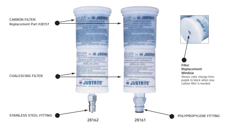
Two-stage filter addresses environmental concerns by capturing 99% of liquid particulates to minimize odor. Filter comes fully assembled and quickly snaps into fitting on can for easy set-up. Top carbon filter with filter replacement window simply twists on to coalescing filter for easy filter changes.
