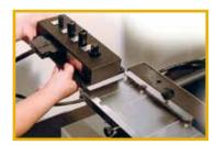
4 in 1 Transducer Slides Easily into Adapter Kit
