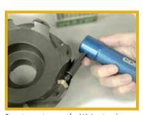
Prevents premature wear of carbide inserts and damage to cutter head due to improper clamp load.
