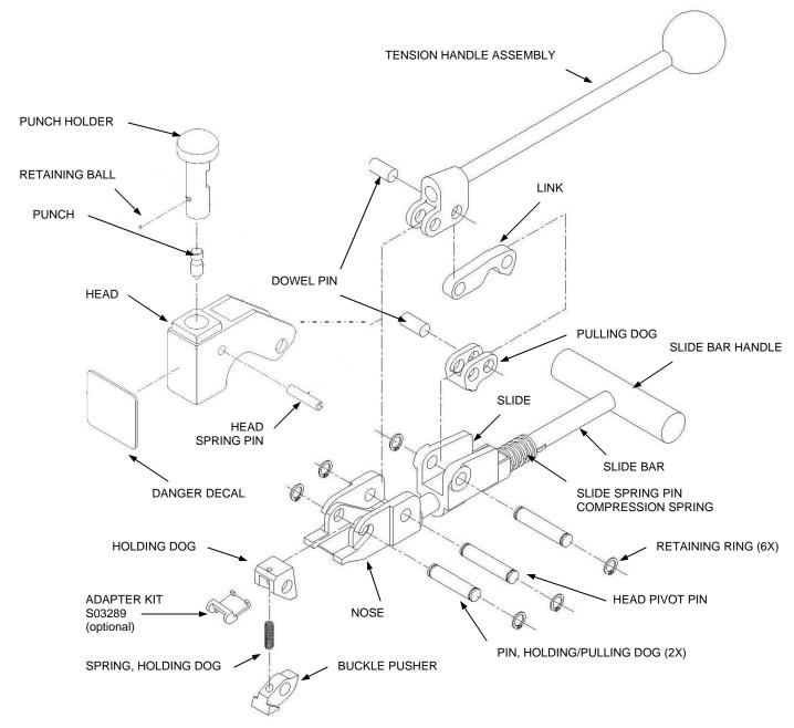
INSTRUCTIONS: DISSASSEMBLY AND ASSEMBLY OF PUNCH
